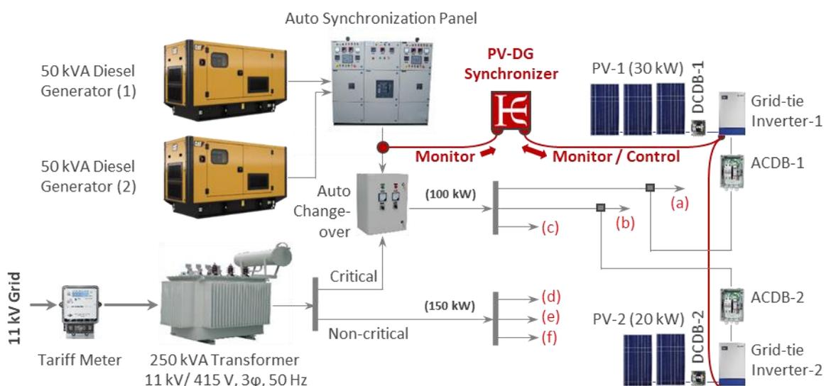
Figure 2: Interconnection for a sophisticated solar-diesel generator synchronization 'solution'.
